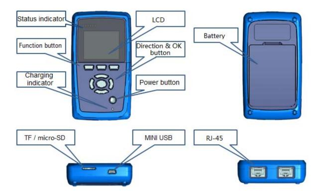
NCT-500 has two RJ-45 ports on the top and has one Micro SD card connector, one Mini USB connector on the bottom. Front have six LED status indicator and one charging indicator. NCT-500 has one 2.2 inch LCD screen, the battery install in the back.
